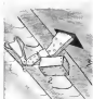
Two small details occur: stabilizer. When flap is extended and stabilizer door closes, gap between fins is closed by rectangular wing block for better streamlining. Slaves are: (1) flap; (2) skin; and (3) stabilizer door.
